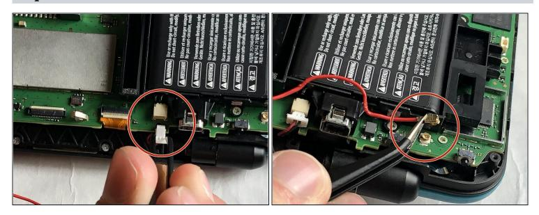
Unplug the following wires from the motherboard using a pair of tweezers.
