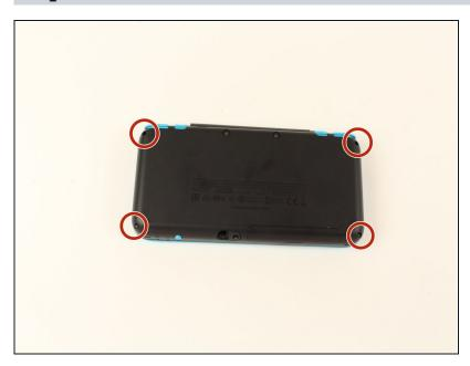
Unscrew the four 6mm tripoint screws located at the four corners of the bottom panel.
