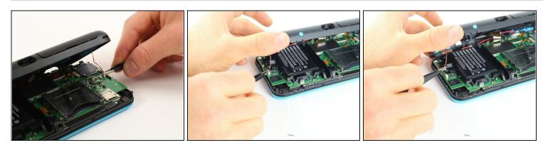
• Using tweezers, disconnect the two cables that connect the rear buttons on either side to the motherboard by gently pulling them upwards.
