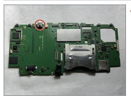
Remove the motherboard and locate the charging port. Flip the the motherboard over.
