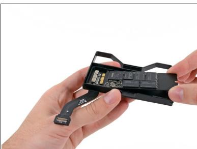
Carefully pull the SSD straight out of its socket on the SSD tray.
