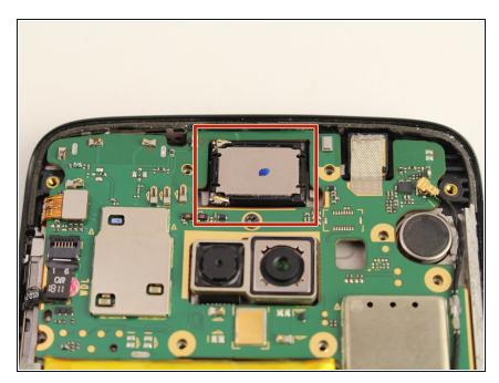
With the interior plate removed, locate the speaker.
