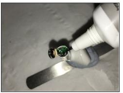
• Finally, the negative electrode of the battery is welded and stabilized with B-7000 glue, but to be more stable, it is recommended to use ab glue or epoxy glue.
