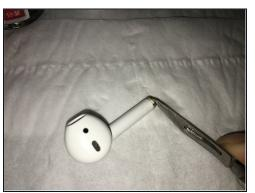
Well, start the official airpods battery replacement and disassembly. After heating, use a scalpel to slide open the bottom charging microphone unit.
