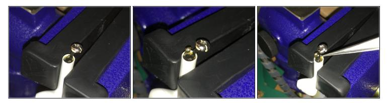
Change direction, continue to tilt the lower cable, and solder the battery positive with a soldering iron.
