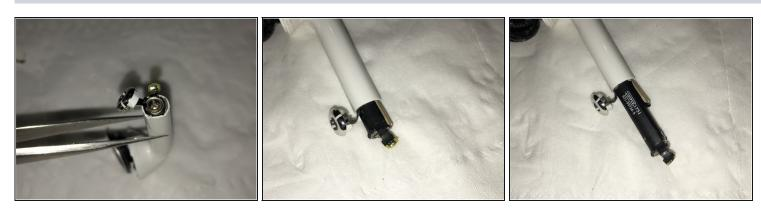
• It can be seen that when the first attempt to practice disassembling the battery, the signal antenna components have been pulled out, resulting in damage to the antenna components.
