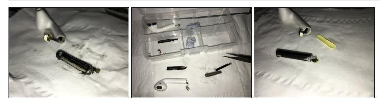
Be prepared to replace the battery removed from the previously damaged airpods, and prepare the sticker on the back of the adhesive to cut the appropriate size.
