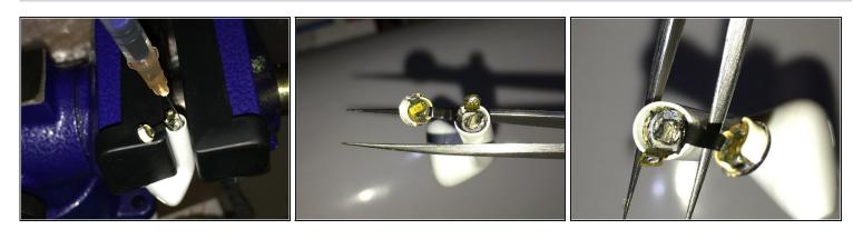
Use a syringe to inject the glue around the outside of the battery, waiting for the rubber foam to soften
