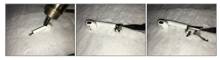
• Finally, heat the upper part around the outer casing of the earphone with a heat gun to soften the filling rubber on the inside. After heating, drip the sol and Zippo again. Finally, use the hook and pliers to slowly pull the battery out.
