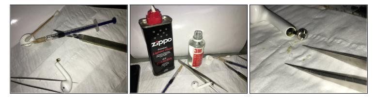
At the same time, the fuel for the Zippo lighter is prepared for the next foaming dissolution, and then the inner glue is cleaned.
