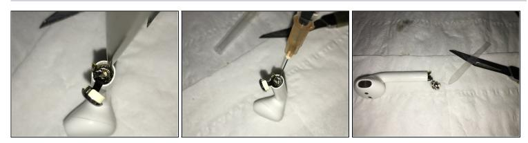
• Use a pair of tweezers to shake the antenna on the outside of the battery to the left and right, then drop the debonding agent, and finally insert a thin plastic piece into the middle of the battery and the inside of the antenna, up and down, to loosen the battery and the antenna.
