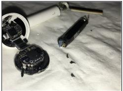
Close-up of the original parts of the airpods after the disassembly of the battery, for the complete disassembly of the bottom to make reference
