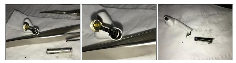
Finally finally the battery is perfectly removed, you can see the bottom of the charging and microphone parts cable and antenna cable in the airpods
