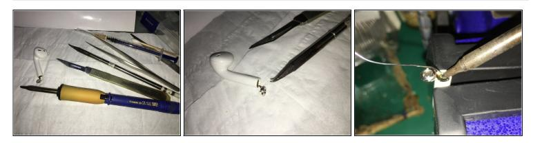
Prepare the required disassembly and soldering tools, fix the airpods, add a small amount of solder for faster heat conduction, and more convenient to remove the bottom battery cable at the bottom.
