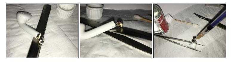
After taking out, pay attention to the internal measurement microphone cable, don't break it, gently open it and drop it into the debonding agent.
