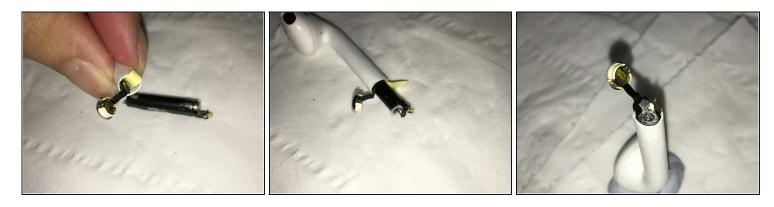
• Insert the cut piece of paper into the middle of the battery cable and the antenna cable to facilitate the battery insertion and to reduce friction.
