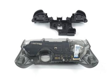
• Remove the trigger buttons from the plastic cover.
