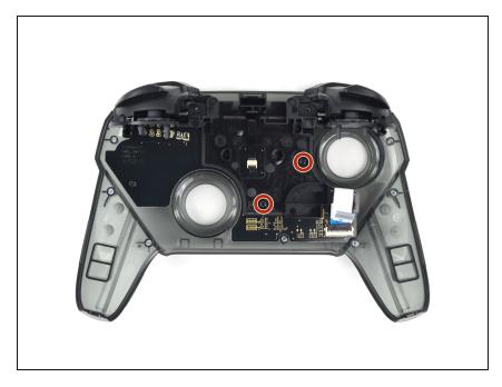
Remove the two 6.8 mm-long screws on the top circuit board using a Phillips screwdriver.
