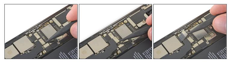
• Use a spudger or a fingernail to disconnect the first two camera cable connectors by prying them straight up from their sockets.
