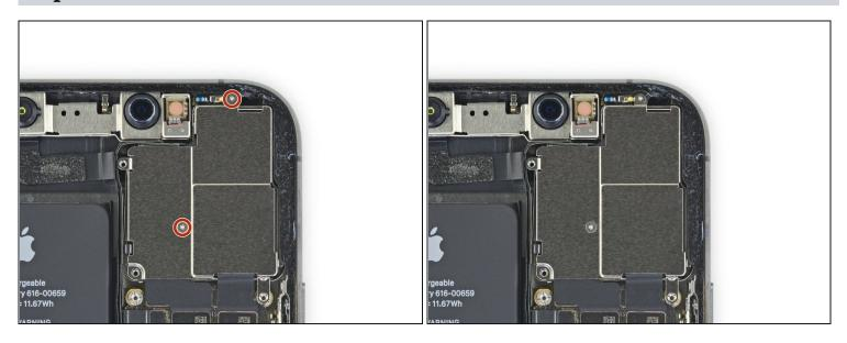
• Use a Y000 driver to remove the two 1.2 mm screws securing the rear camera cover.
