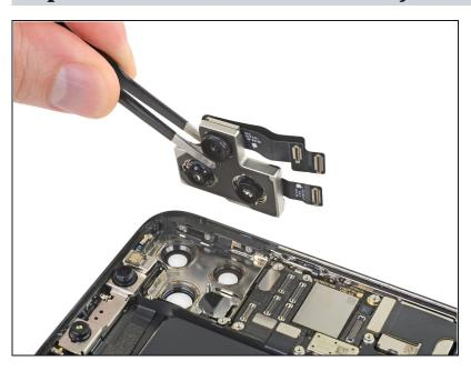
Remove the rear-facing camera assembly. Compare your new replacement part to the original part—you may need to transfer remaining components or remove adhesive backings from the new part before installing.
