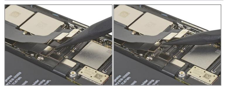
• Use a spudger to disconnect the third camera—its connector lies underneath the cable you disconnected in the previous step.
