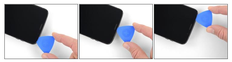
• Slide your tool underneath the top bezel to separate the glue.
