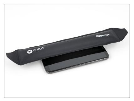
Heat the left edge of the phone to soften the adhesive securing the left edge of the display.
