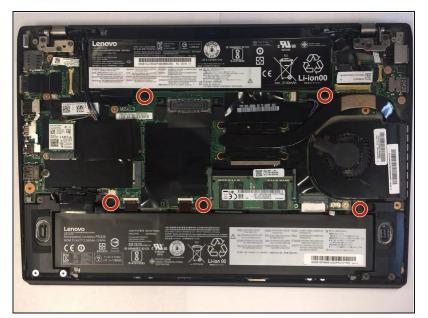
Remove the five 5.5mm Phillips #1 screws securing the two batteries.
