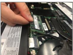
• To remove the existing RAM module, pull tabs marked in the red outwards.
