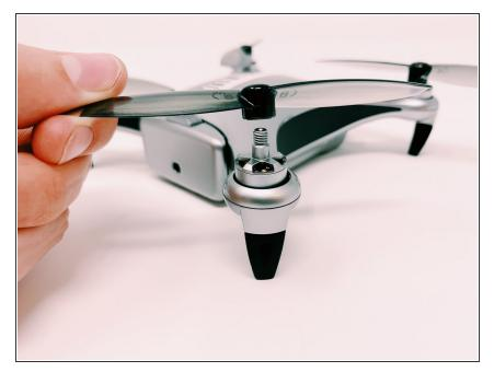
Once you unscrew the propeller from the drone you will then be able to inspect the area for any additional damages.
