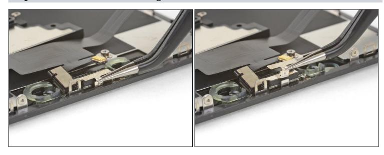
• Use tweezers to slide the small bracket straight up and off of the ambient light sensor.
