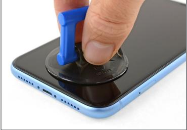
If you're using a single suction handle, apply it to the bottom edge of the phone, while avoiding the curved portion of the glass.
