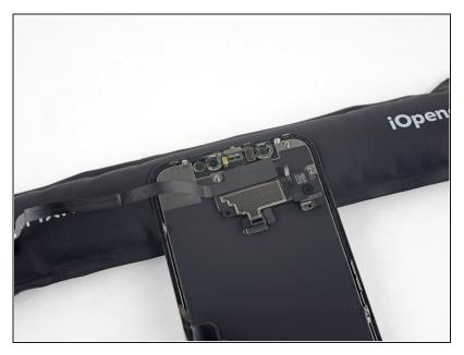
Use a hairdryer, a heat gun, or a heated iOpener applied to the top front of the display for about a minute, in order to soften the adhesive securing the sensors.
