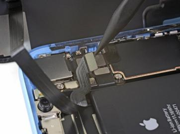
• Use the tip of a spudger to pry the front sensor assembly connector up from its socket.
