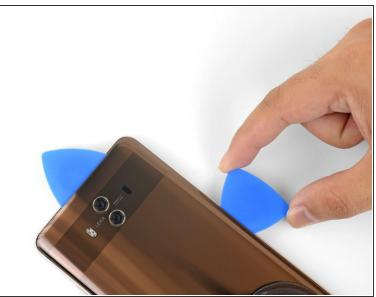
Continue heating and slicing through the remaining edges, leaving opening picks in the seams to prevent the adhesive from re-sealing.
