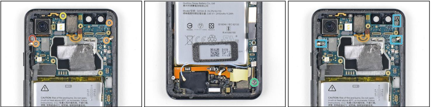
**i** Some of these screws hold very small grounding clips in place. *Be careful not to lose these clips* as you remove the screws.
