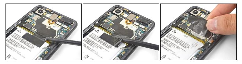
⚠ Whenever you use the spudger near the battery, be very careful not to puncture the battery.
