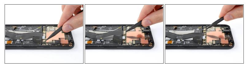
• On the other end of the battery, pry up and disconnect the other side of the interconnect cable, as well as the two squeeze sensor cables on either side of it.
