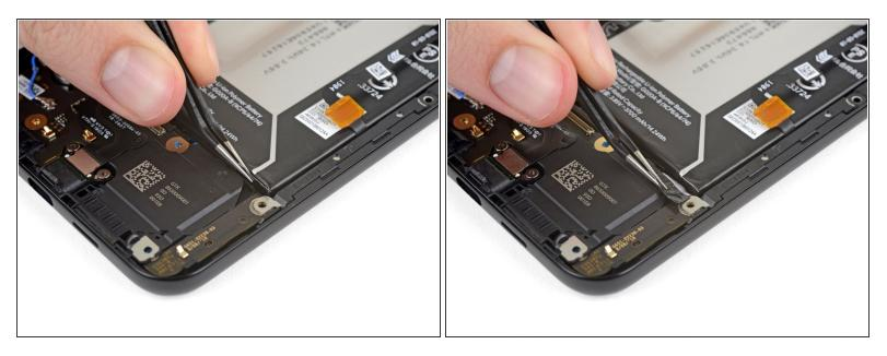
• Use tweezers to carefully pull out the right adhesive strip's pull-tab from the bottom right corner of the battery.
