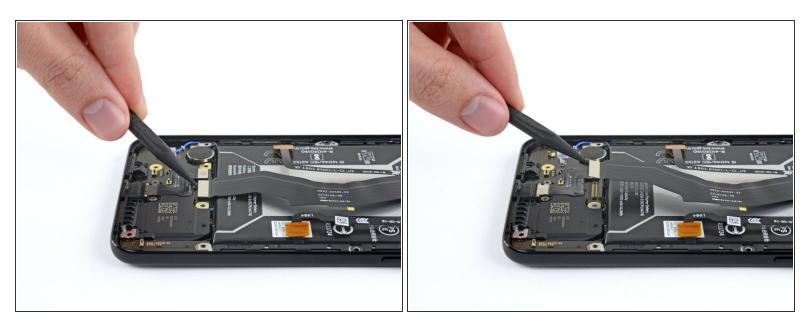
• Use the pointy end of a spudger to lift up and disconnect the lower half of the thick board interconnect cable that runs over the battery.
