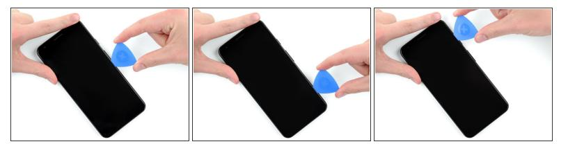
• Once the pick is inserted, slide it up and down along the right edge of the phone to cut though the adhesive holding the screen in place.
