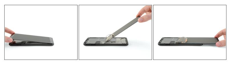
• Lift the screen by its top edge (where the front-facing camera is) and carefully flip it 180° so that the screen is resting face-down on the phone.
