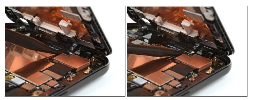
• Use a spudger to pry up and detach the proximity sensor cable from the motherboard.
