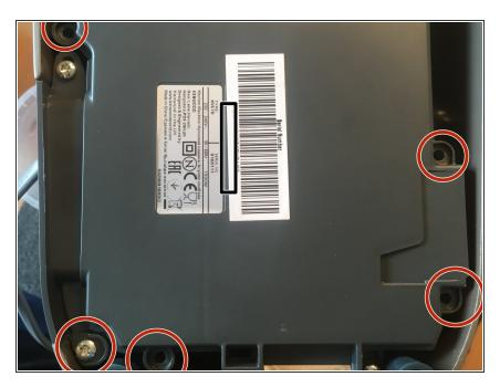
• Remove five Screens T20 from the bottom and lift the bottom plate up.
