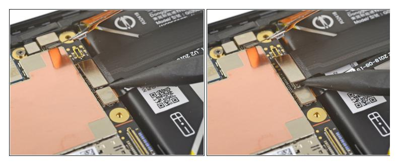
• Use the point of a spudger to pry up and disconnect the interconnect cable from its motherboard socket above the battery.
