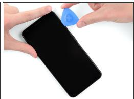
Once the pick is inserted, slide it up and down along the right edge of the phone to cut though the adhesive holding the screen in place.
