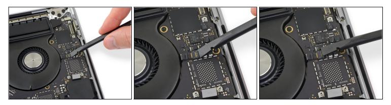
• Open the locking flap on the microphone cable's ZIF connector by prying it straight up from the logic board.
