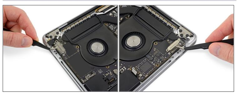
• Remove the cover brackets from both Thunderbolt cable sockets.
