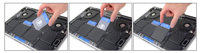
• Retrieve your second plastic card and repeat the previous step to separate the remaining center battery cell.
