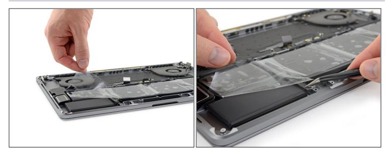
• After your battery is properly positioned and installed, peel off and discard the clear plastic liner from the top.
