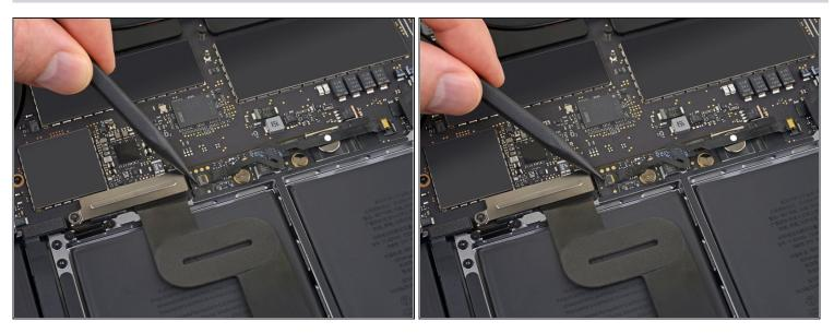
• Pry up and disconnect the locking flap on the connector at the opposite end of the battery board data cable.
