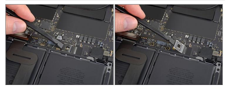
Use a spudger to lift the battery power connector, disconnecting the battery.
