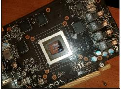
Wipe the top of the graphics chip gently with 91% isopropyl alcohol to remove the old thermal paste, avoid being too rough to prevent scratching the chip.
