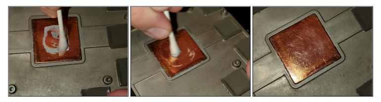
• Repeat that process on the heatsink. This will allow for even distribution of the thermal paste to fill properly.
