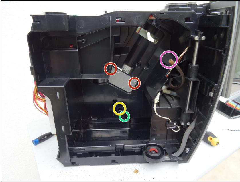
**i** In this image the brewing unit has been removed already to show you how it is connected.
