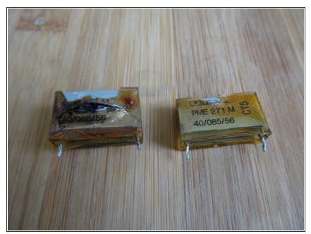
Here is a picture of the two oil paper capacitors. They break more easily, the case cracks. Replace them with more modern MKP types.
