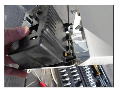
Take out the motor cover. It is held under the axle of the pedestal.
