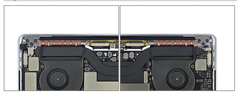
• Use a P2 Pentalobe driver to remove the sixteen 1.5 mm screws securing the antenna assembly.
