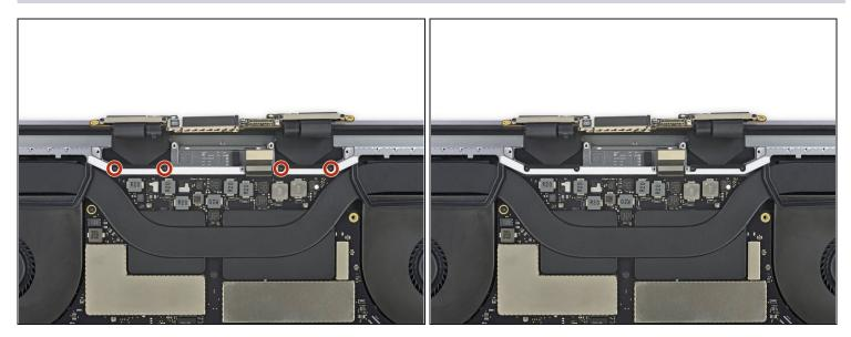
Use a T3 Torx driver to remove the four 3.9 mm screws securing the display cable cover springs.
