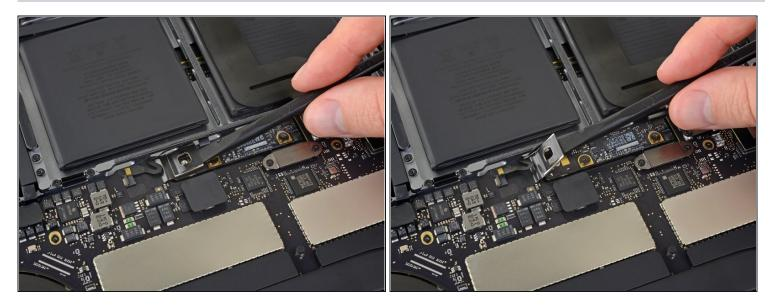
Use a spudger to gently lift the battery power connector, disconnecting the battery.
