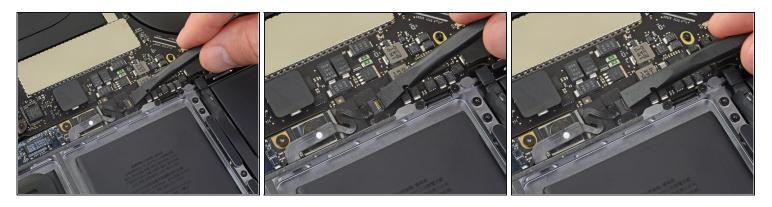
• Use a spudger to gently pry up the locking flap on the <u>ZIF connector</u> for the battery board data cable.
