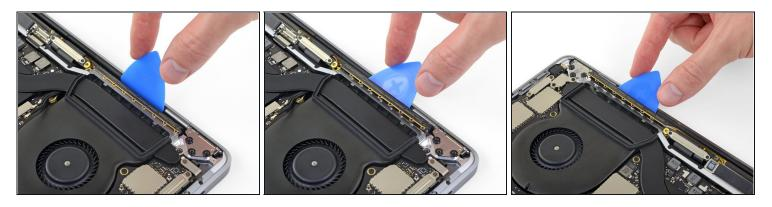
• Use an opening pick to pry up the antenna assembly and separate it from the MacBook Pro.
