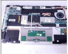
With the backplate and battery removed from the device, remove the three 2mm screws using the Phillips #0 screwdriver.
