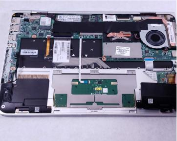
• With all three screws removed, remove the speaker assembly from the device.
