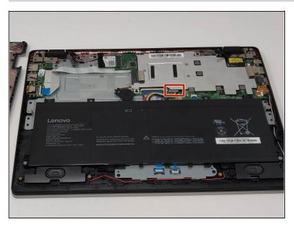
For safety reasons, disconnect the wires connecting the battery to the motherboard with a nylon spudger.
