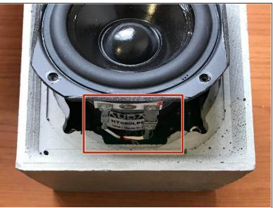
• Connect the speaker as in step 3. Take care to ensure the connectors are on the side where there is a notch in the concrete.
