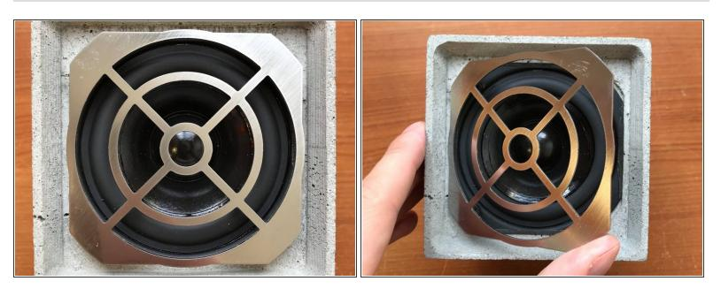
Remove the speaker protective grill by first lifting one corner.
