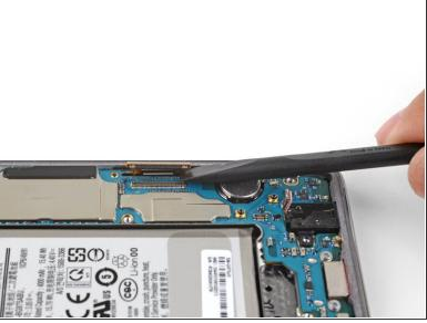
Use the flat end of a spudger to pry up and disconnect the display connector from its motherboard socket, located near the bottom right corner of the phone.
