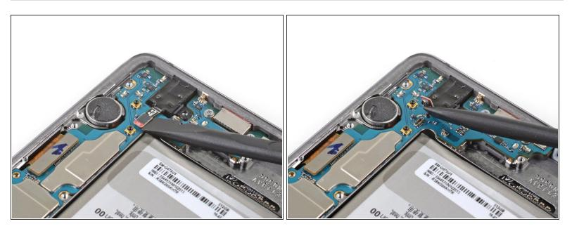
Use the flat end of a spudger to pry up and disconnect the headphone jack's connector from its motherboard socket.
