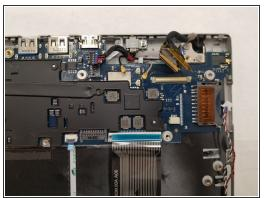
• The screen cable is secure in place by a lever. Lift the lever to release it, then gently pull it out.
