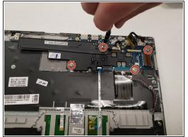
• Unscrew the four 3.1 mm screws holding the motherboard with a Phillips #00 screwdriver.
