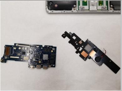
• Finally, remove the three 3.1 mm screws with the Phillips #00 screwdriver to remove the plastic cover and completely free the motherboard.
