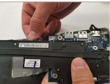
Lift the motherboard out of place and pull out the CMOS battery cable.
