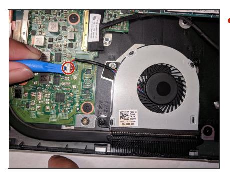
Use a plastic opening tool to unclip the connector that attaches the fan to the motherboard.
