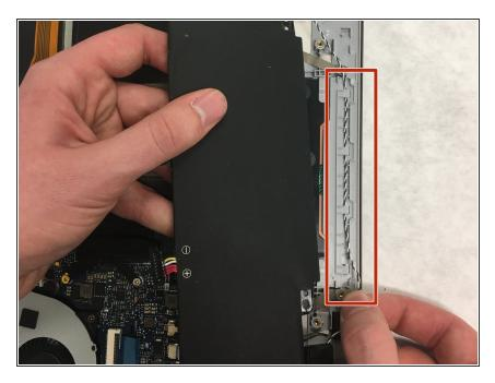
Deroute the speaker cable from the clips so the battery can be fully removed.
