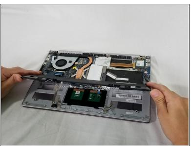
Lift up and remove the battery and speakers from the device.
