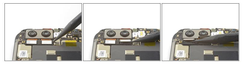
• Use the point of a spudger to pry up and disconnect the two rear-facing camera connectors from their sockets on the motherboard.
