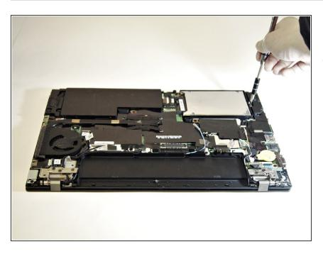
• Unscrew the single screw that holds the hard drive in place.
