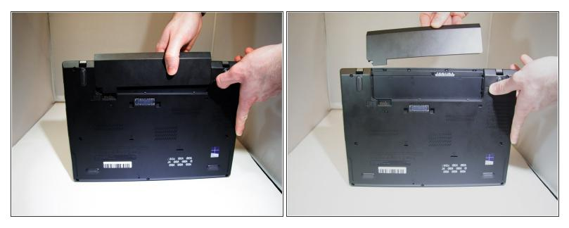
• Slide lock button 2 to the unlock position and continue gently sliding until the battery is removed.
