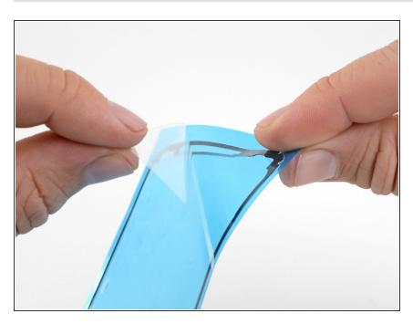
Peel the clear backing layer off of the replacement adhesive.
