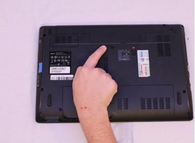
Flip the second slider to its unlocked position.
