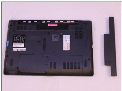
Remove the old battery pack from the device and insert the new pack.
