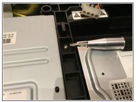
Now you need to remove 2 cords. The power cord can be tricky. Remove 1 screw using a T 10 screwdriver.
