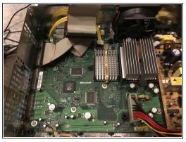
You should lift the hard drive. Remove 2 cords and remove 2 screws. After removing the disk drive, you've made it to the motherboard.
