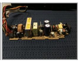
Now remove this cord and remove the 2 screws holding the power supply. Yup that's the power supply.
