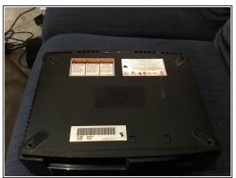
First you need to remove 6 screws using a T 20 screwdriver. Two are hidden in 2 stickers.
