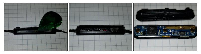
Using a small pick or pry tool, separate Receiver Housing. Each side is secured by 3 small fragile tabs. Use the space near the micro USB opening & carefully pry to separate the 3 tabs on the opposite side.
