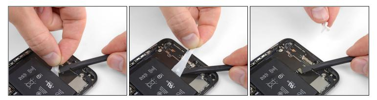
Remove the center strip, being very careful not to snag it on the speaker flex cable.
