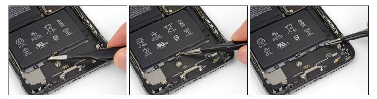
• Repeat the above step to separate the remaining two adhesive tabs from the bottom edge of the battery.
