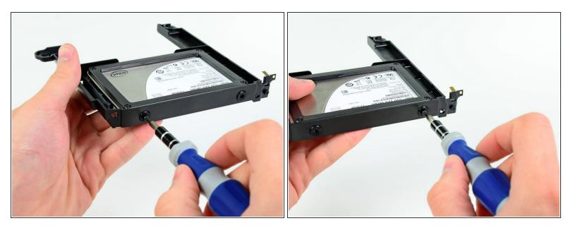
Use a T6 Torx screwdriver to install the remaining two set screws through the grommets and into the side of the hard drive.
