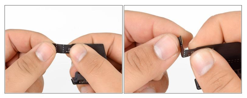
• Hold the ribbon cable on either side of the first small dotted line and bend it up 90 degrees.
