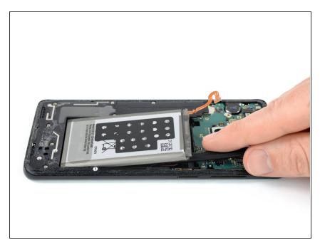
Insert the spudger at the top right corner of the battery and pry it up.
