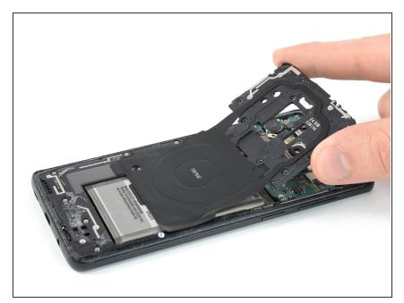
Remove the plastic cover containing the NFC antenna and the charging coil.
