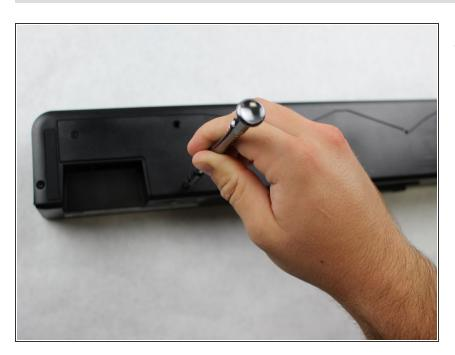
Remove five 18.25mm screws with a Phillips #2 screw driver.
