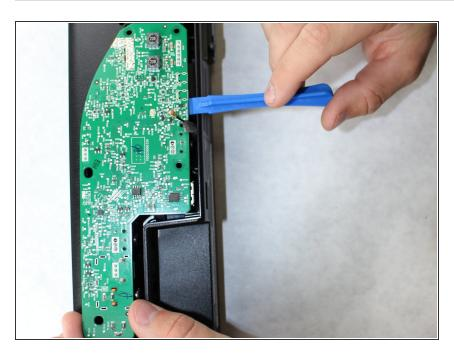
Using the plastic opening tool, slightly lift the circuit board up and remove it from the housing.
