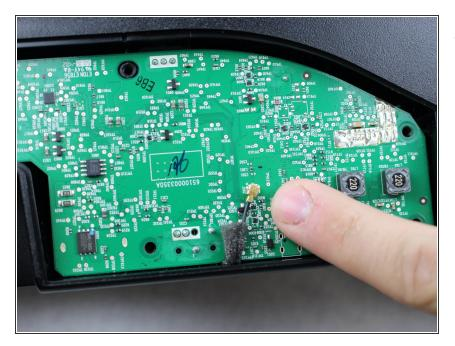
Gently remove the gold plates and the snap connector from the circuit board by pulling it apart.
