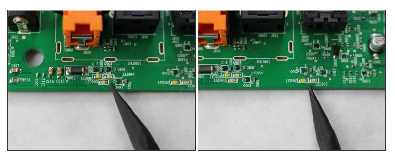
Locate on the back of the control panel where it states LED 902, 903, 904, and 905.
