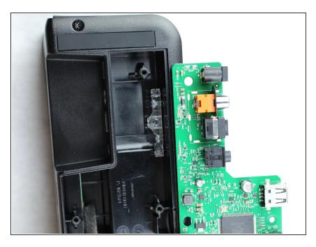
Locate the two clear LED receptors and note that one has two prongs and the other has three prongs.
