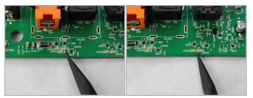
• If there is any debris located in these locations, use the spudger tool to thoroughly clean the area.
