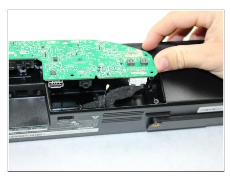
Disconnect the cords running to the white connector by pulling upon the tab until it is disconnected completely.
