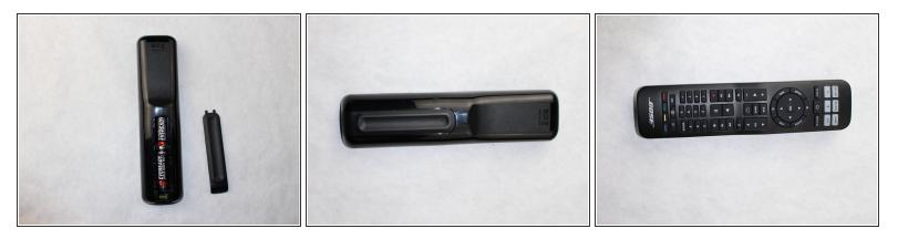
• To reassemble your device, place the cover back over the batteries by lining up the teeth and sliding upward until you hear a click.
