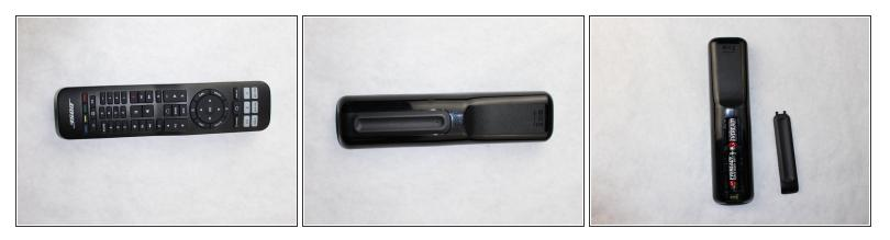
• Open the battery compartment cover on the back of the remote by applying pressure with fingers and sliding downward.
