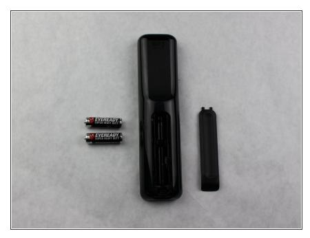
• Remove both AA batteries carefully.
