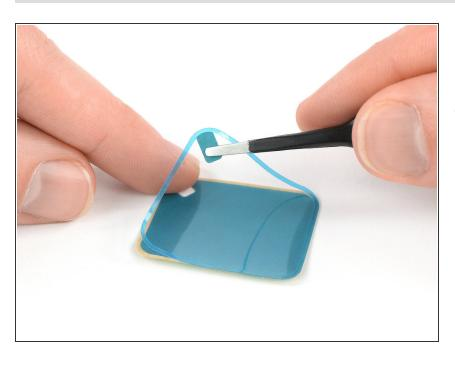
Use a pair of tweezers to carefully remove replacement adhesive with the blue protective film from the backing paper.
