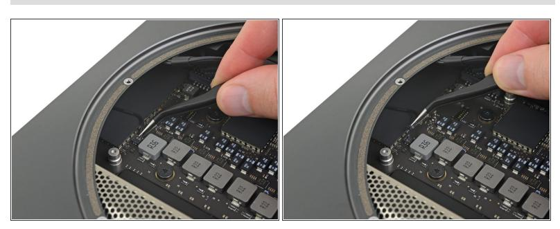
Carefully lift the connector for the LED indicator light straight up to disconnect it from its socket on the logic board.
