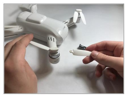
Remove the propeller by pulling it out.
