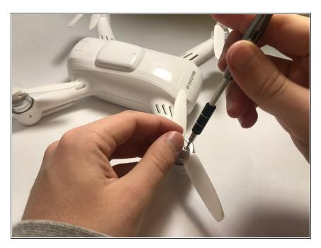
• Take out the screw using the H1.5 allen bit.
