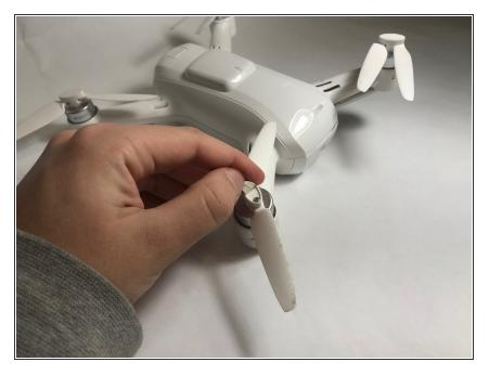
• Lift the foam piece on the top of the propeller.
