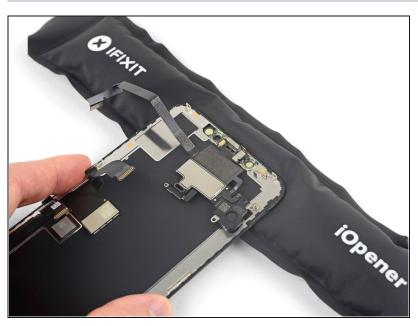
Use a hairdryer or heat gun or prepare an iOpener and apply it to the top front of the display for 1-2 minutes, in order to soften the adhesive securing the sensors.
