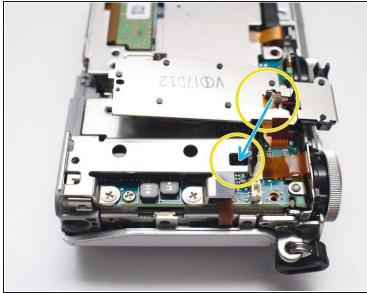
Insert small crowbar or flat head screw driver here to lift the keypad up.
