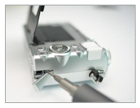
Remove 1 screw under the DC power cable notch cover
