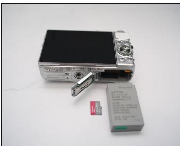
Remove Lens, MicroSD Card and Battery
