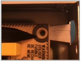
Here's a better view of the plastic piece with the board removed. You're just squeezing the two little "wings" together while pulling up on the board. Be patient, it can be a little tedious.
