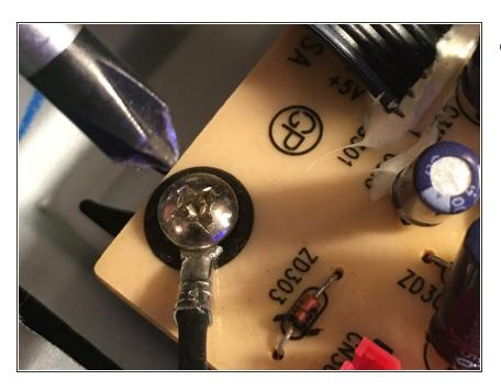
Reassembly is the reverse of the disassembly process. Don't forget to reattach the ground wire under the screw that secures the board.
