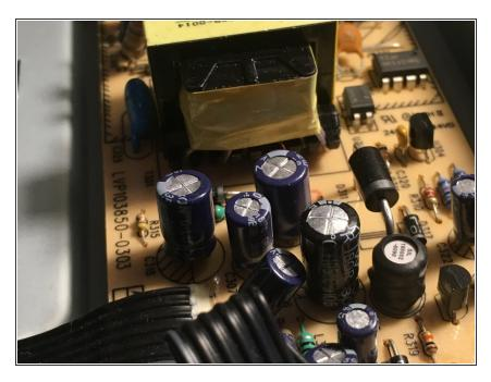
Take care not to touch any of the components on the Power Supply Board. There could still be high voltage present.
