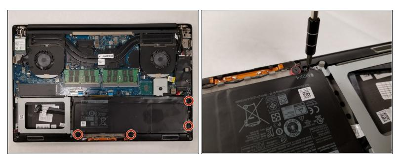
• Remove the four 4.0 mm JIS #0 screws surrounding the battery.
