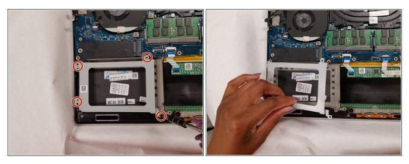
• Remove the four 4.0 mm screws with a Phillips 1 screwdriver, and remove the hard drive bracket.
