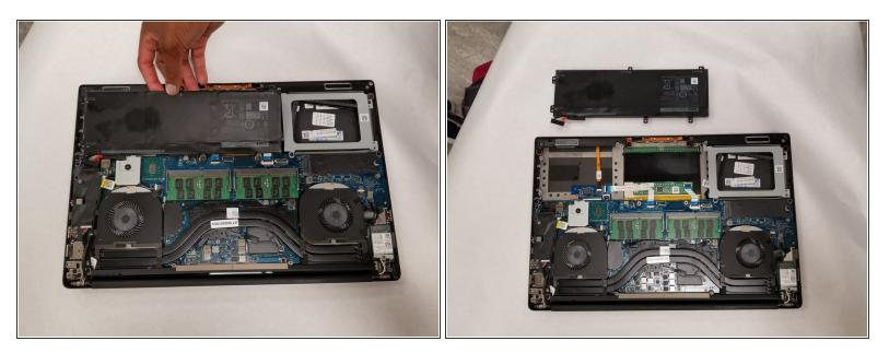
• Carefully remove the battery from the computer.
