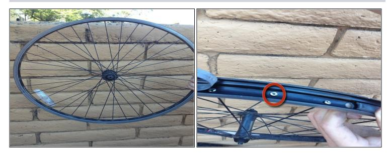
Slowly peel back the layer of rubber that covers the 32 screws on the wheel.
