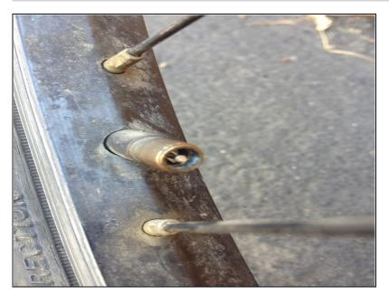
Locate the valve stem and remove the valve stem cap if one is present.
