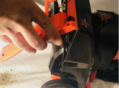
• Lift off the brush plate by grabbing both ends of the plate and lifting the plate up.
