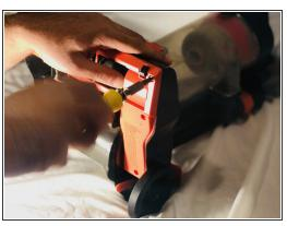
Remove the 5 screws from the brush plate with the phillips screwdriver.
